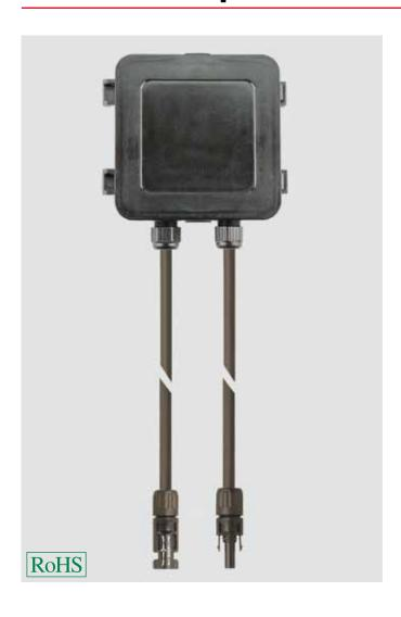
Suitable for connecting SOLARFLEX®-X PV1-F cables to the core cross-sections 2.5 mm², 4 mm² and 6 mm². With two bypass diodes. Preventing condensation using a bronze air filter. A set of adhesive elements are included for tight and lasting mounting on any solar module.
